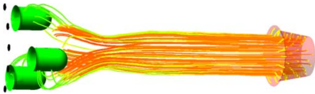
Fig. 7 Visualization of current density (red = high, green = low) in-between the three cathodes and the anode ring with Lorentz force
